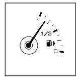
The fuel gage shows approximately how much fuel is in the fuel tank. It works only when the ignition is in the ON/RUN position.
